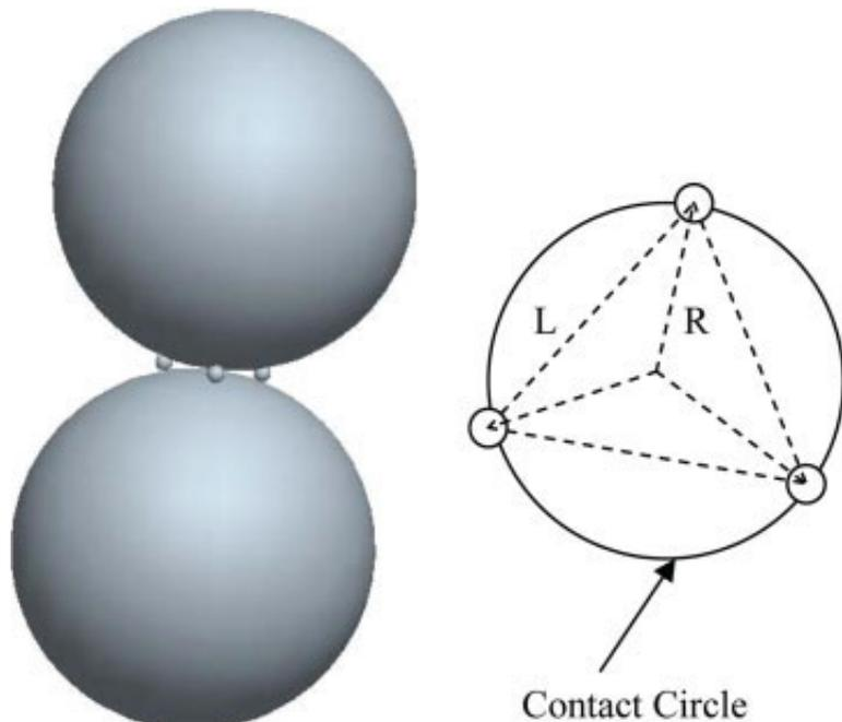
$$F_{ad} = \frac{Ad}{4z_0^2} + \frac{A}{24 \left( \sqrt{\left(1 + \frac{d}{D}\right)^2 - \frac{1.21}{SAC} \left(\frac{d}{D}\right)^2} - 1 \right)^2 D}$$
