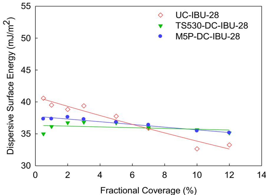
**Fractional coverage:** how much surface area of the powders being tested; different amount of solvent probe is injected in the IGC
