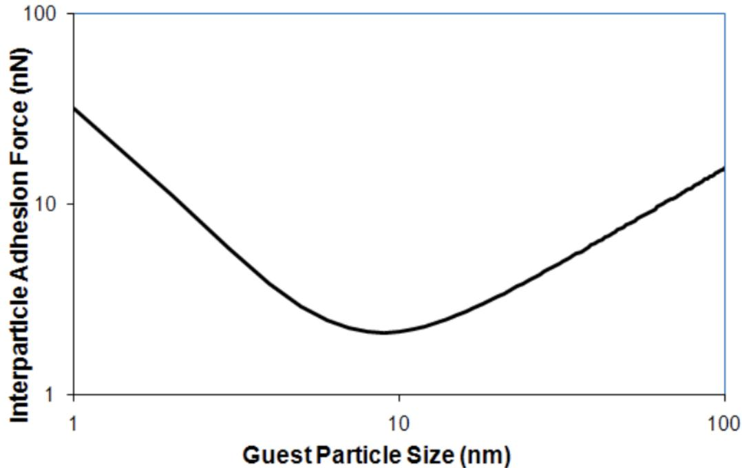
An **optimal** guest particle size leads to the minimum interparticle adhesion force (left)
