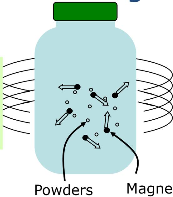
Oscillating Electromagnetic Field, causes magnets to spin at up to 1000 Hz
