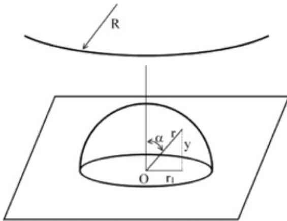
$$F_{ad} = \frac{A}{12z_0^2} \left[ \frac{dD}{d+D} + \frac{D}{(1+d/2z_0)^2} \right] \quad \text{Rumpf Model – Single asperity}$$
