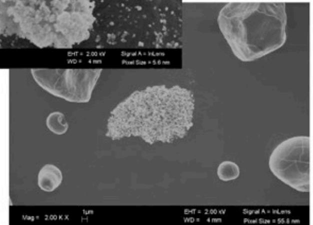
MAIC/Dry Coated versus V-Blended (for relatively easy host particles)
