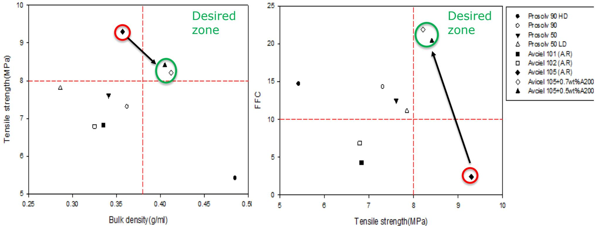
Compared with commercial excipients, the surface engineered excipients exhibit better performance in bulk density, flowability as well as compaction shown in these phase maps
