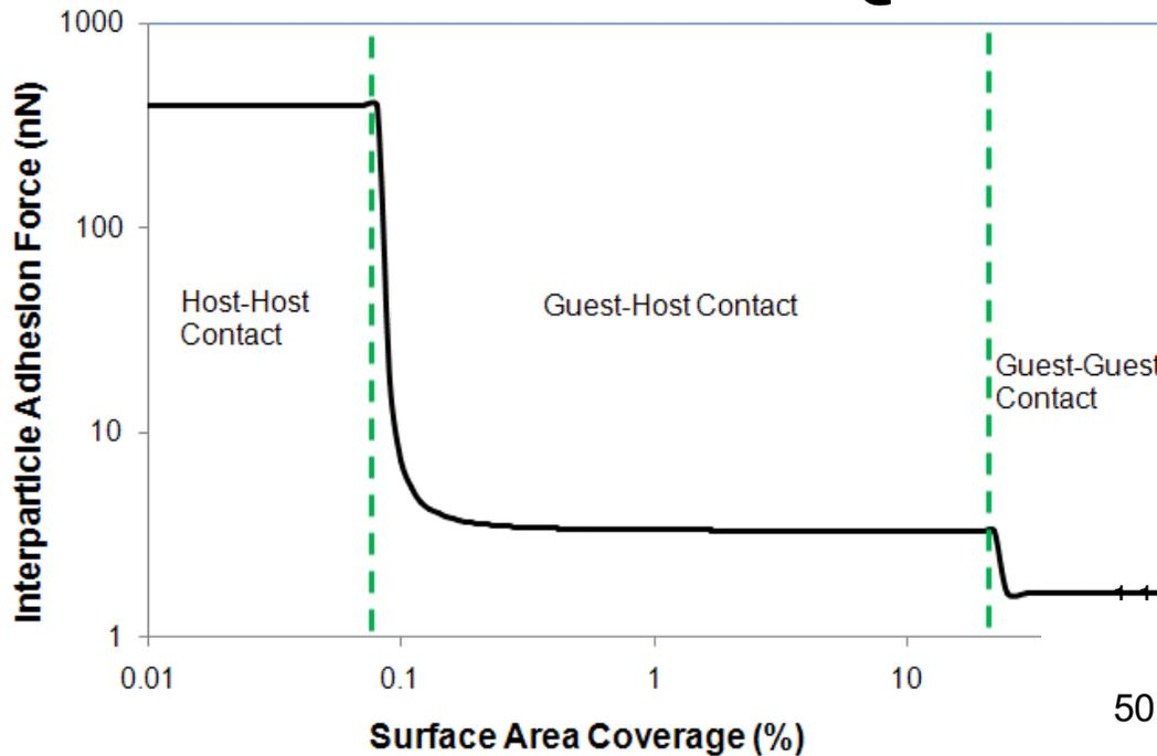
Contact Mode/SAC significantly affects the inter-particle force and fluidization behavior
