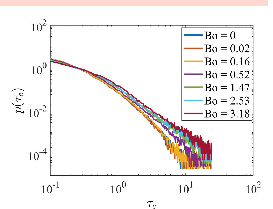
Cohesion increases number and and duration of contacts. Must use data on micromechanics to build a continuum model.
