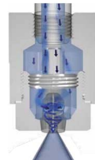
Swirl Nozzle with Tangential Inlet
