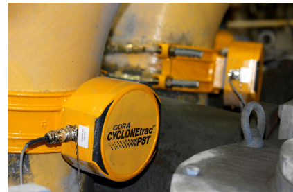
CiDRA PST mounted on hydrocyclones (cidra.com)
