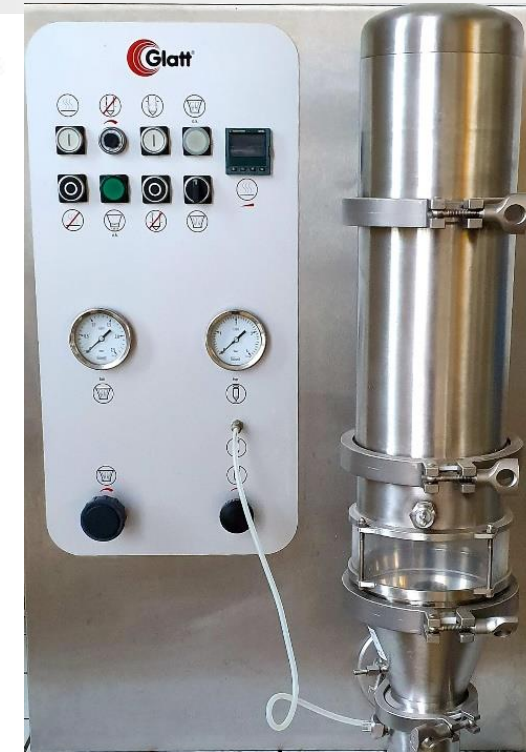
Mini-Glatt fluid bed coater (Würster design)
