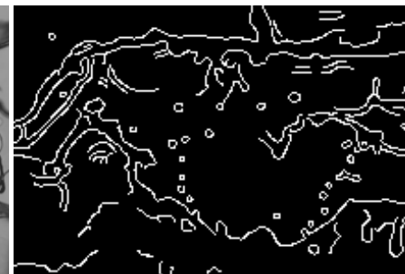
Imaging & image processing to determine droplet sizes and ligament thicknesses.
